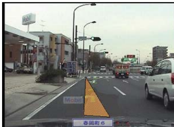
Fig.13 Superimposed indication of a head-up display (HUD)
