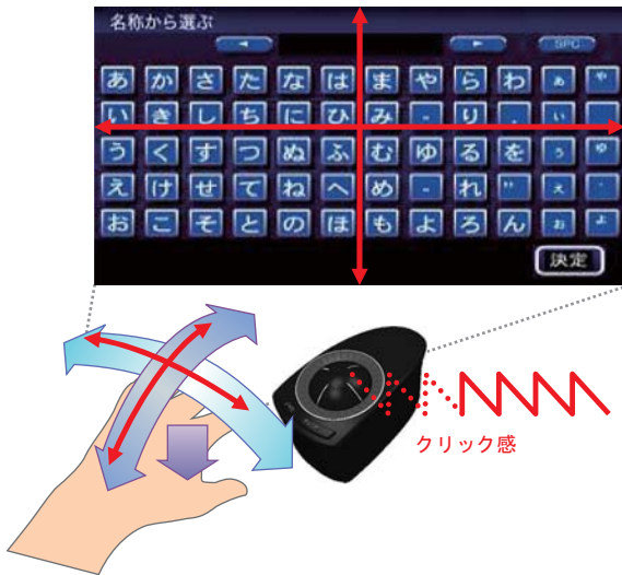
Fig. 14 Remote touch controller with haptic feel
