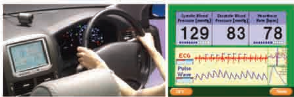
Fig. 11 Daily health check system. This figure shows one of the potential applications of our steering wheel sensor. The system automatically measures and stores a driver's vital signs, and reports the driver's condition as well as any potential risk to the driver's health, and will also summon rescue if necessary.
