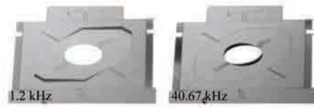
Fig. 9 View of the scanning motion observed under microscope and LED pulse light source
