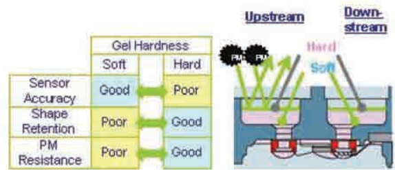
Fig. 9 EGPS Structure to withstand Environment
