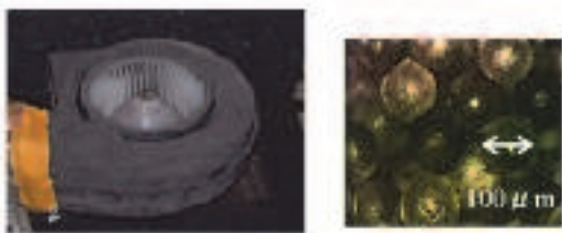
Fig. 20 Sound permeable scroll casing
