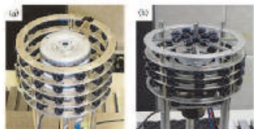
Fig. 6 Cylindrical microphone arrays (a)For inner rotor motor (b)For outer rotor motor
