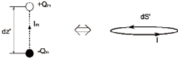
Fig. 7 Magnetic dipole and electrical current loop
