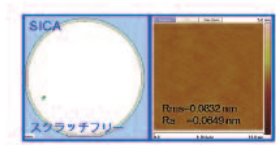
Fig. 9 Entire surface evaluation of wafer using confocal differential interference microscope (C-DIC) and surface roughness evaluation using AFM
