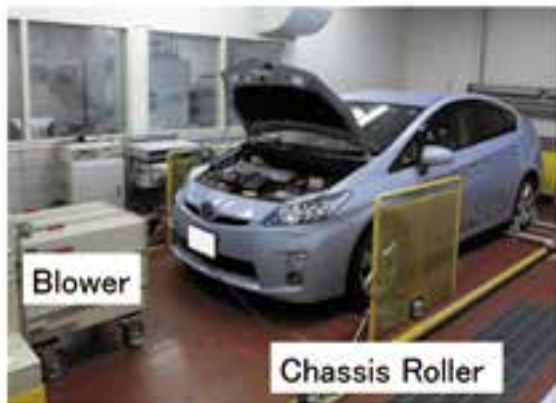
Fig. 4 Vehicle Test using Chassis Dynamometer
