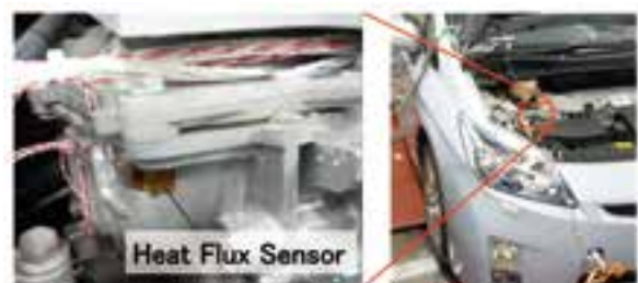
Fig. 7 Sensor Installation to the Engine (Sample)
