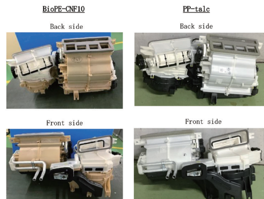
Fig.14 Evaluated air conditioner case assembly
