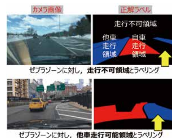
Fig.4 Labeling variability for the same class: examples from the BDD100K Dataset [Yu 18]
