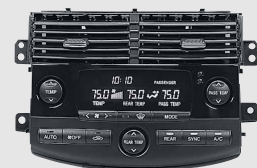
INTEGRATED CLIMATE CONTROL PANEL
